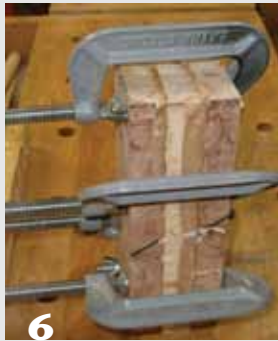
6 The assemblage is glued and clamped. Let the glue cure overnight.
