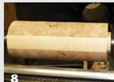
8 Turn the assembly to a cylinder and turn a tenon on one end.
