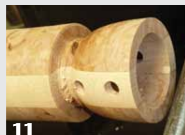
11 Hollow the inside of the goblet cup.
