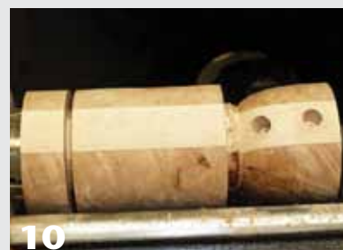
10 Drill holes into waste wood for checking thickness (if desired).
