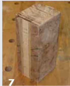
7 Cut away enough wood from each end to eliminate the alignment holes.
