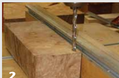
2 Drill alignment holes in the goblet blank before resawing.
