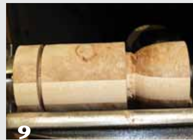
9 Mark where the foot and goblet will be, then shape the goblet cup.
