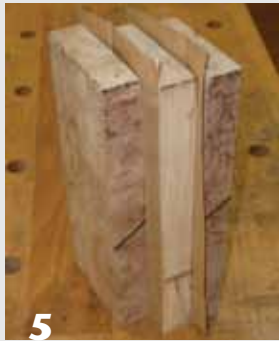
5 The entire assemblage, including the paper layers, is ready to be glued.
